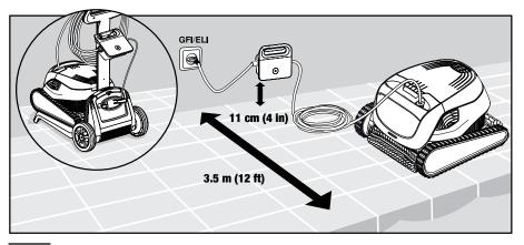
5.1.1 Position the power supply so that it is approximately in the middle of the long side of the pool at a distance of min 3.5 m (12 ft) from the pool and placed 11 cm (4 in) above ground.
