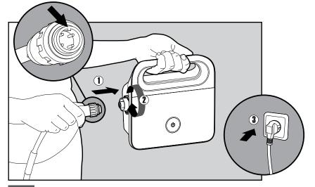
**5.1.3** Attach the floating cable to the power supply by inserting it with the notch on the connector (1), lined up with the groove in the socket on the power supply, and turning clockwise (2). Plug in the power supply and leave it in the OFF position (3).
