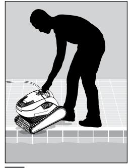
5.4.3 Place the Pool Cleaner on the edge of the pool and let the water drain out.
