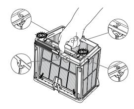
6.2.5 Assemble the filter panels according to the following order: Panel  $4 \rightarrow 3 \rightarrow 2 \rightarrow 1$ .
