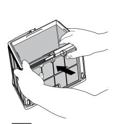
6.2.2 Dismantle the panels, starting by pressing on panel 1 using your thumbs.
