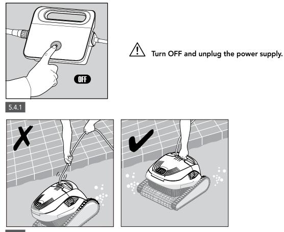
5.4.2 Using the floating cable, bring the Pool Cleaner to the pool's edge. Using the handle, remove the Pool Cleaner from the pool.
