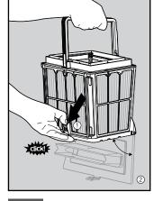
6.1.4 Open the latch to release the bottom lid in order to remove the debris.
