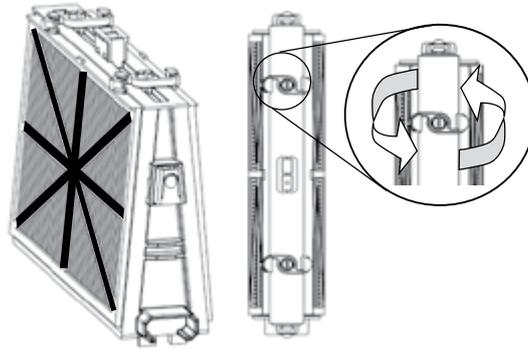
Reinstall the filters according to the diagram
