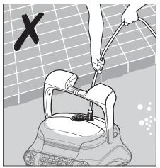
7.4.3 Place the Pool Cleaner on the edge of the pool to let the water drain out.
